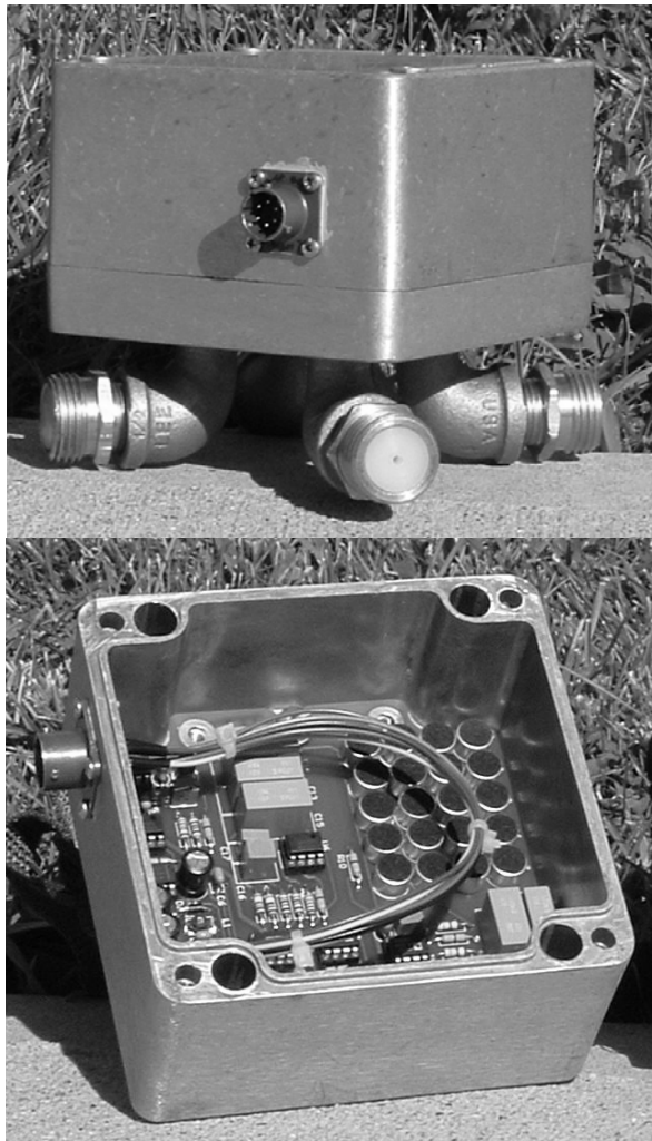
Figure 14. Prototype Avalanche Infrasonic Sensor
